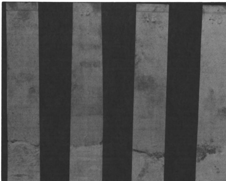
Figure 2. Solder test specimens; two-inch immersion for five seconds.
